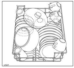
The cup-rack on the left folds upwards to increase your loading flexibility.
